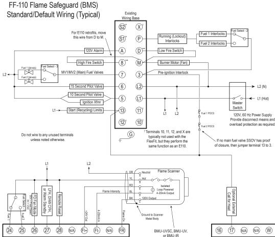
\*Note: Disconnect any existing wires from terminals S1 and S2; they are not used.
